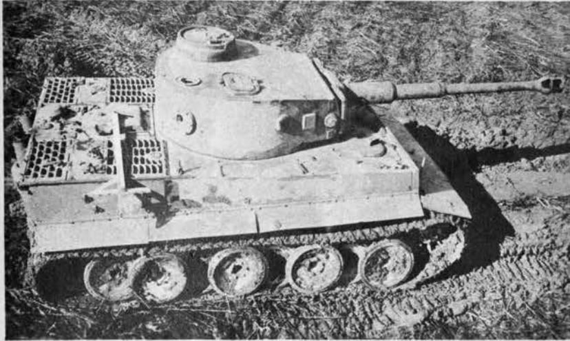
Muscleman of Nazi tanks is the Mark VI, or Tiger, which has a huge cylindrical turret housing its 88-mm. gun. Turret top slopes toward the gun mantlet, ends in a wide flat face. The rear stowage bin is absent in this picture.
